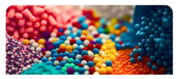
PPA (Polyphthalamide) masterbatches are high-performance additives used to enhance the properties of plastics. These masterbatches are known for their excellent thermal stability, superior chemical resistance, and outstanding mechanical strength. They are widely used in automotive, electrical, electronics, and industrial applications, where durability and reliability are crucial.
